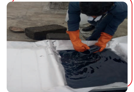
Dissolved sodium sulphate waste is mixed with activated carbon
